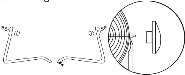
In doing so, connect the ends of the pipe together and secure them with the Phillips-head screw provided. Then mount the nuts using the spanner provided.
