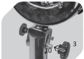
Then secure the motor unit with the lock nut (3) and the carriage bolt (10).
