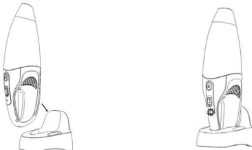
Slide the "On/Off" switch in the direction of "I" to switch it on. Slide the switch to the "0" position to switch it off.
