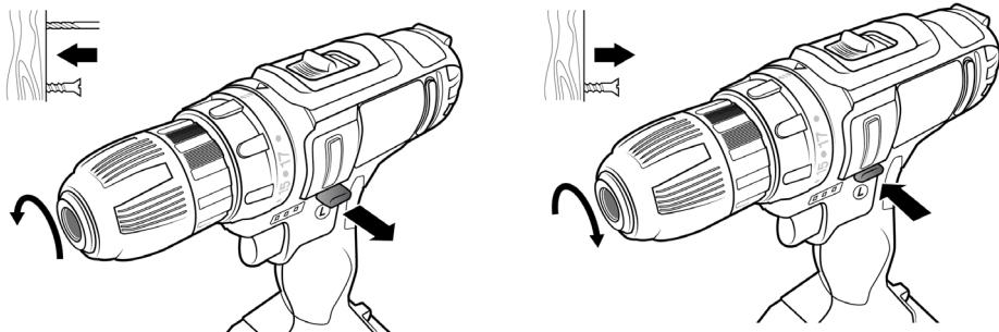
Using the direction change switch, you can change the direction of rotation of the cordless screwdriver as desired.
