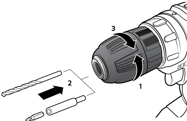
Open the chuck by rotating it (1). Insert the desired screwer or drill bit (2) and tighten the chuck again (3).
