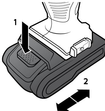
Unlock the battery by pressing the "Battery unlocking" button (1) and then slide the battery out of the device (2). To insert a new battery, slide the battery into the cordless screwdriver on (2) until it locks into place.
