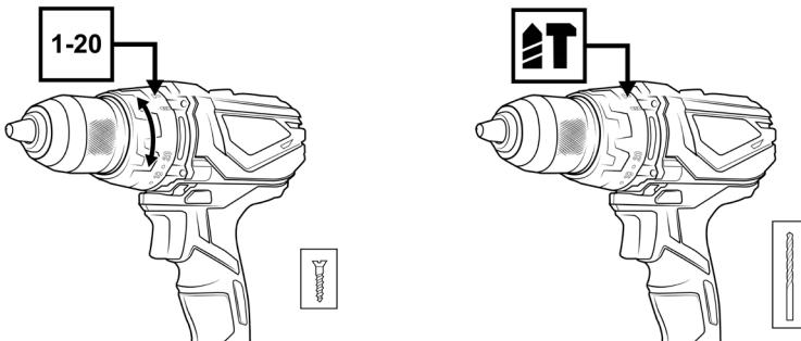
Select the desired torque and set it using the "torque-adjustment ring". Here "1" is the lowest and "20" the highest resistance. If you want to drill, select the drill symbol where there is no torque limit. The hammer icon activates the impact function.
