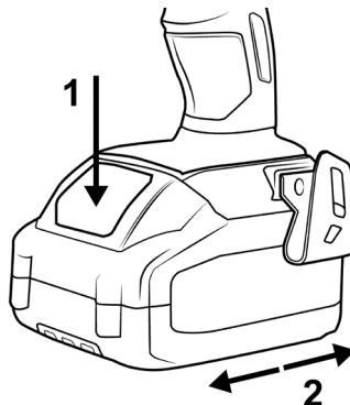
Unlock the battery by pressing the "Battery unlocking" button (1) and then slide the battery out of the device (2). To insert a new battery, slide the battery into the cordless screwdriver on (2) until it locks into place.
