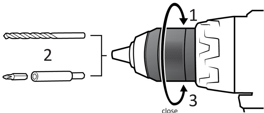
Open the chuck by rotating it (1). Insert the desired screwer or drill bit (2) and tighten the chuck again (3).
