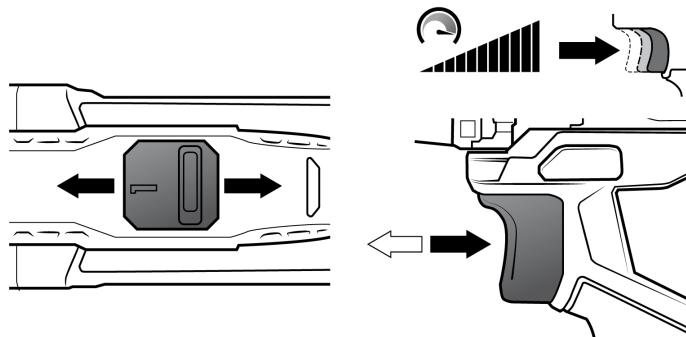
Select the desired speed using the "Speed level switch".
