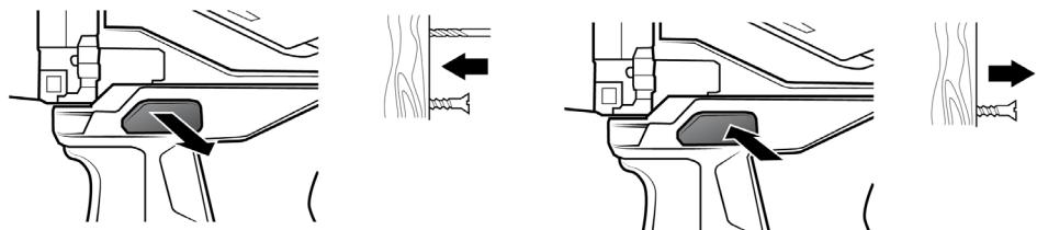
Using the direction change switch, you can change the direction of rotation of the cordless screwdriver as desired.
