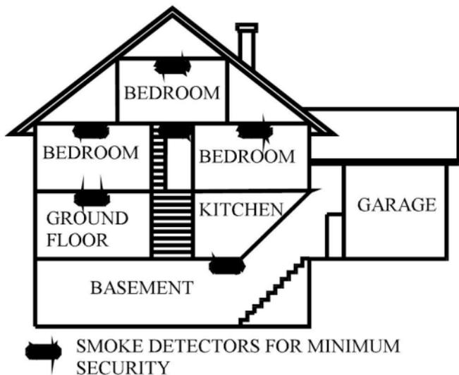
10. Make sure that doors or other objects do not block the path of smoke to the detector.
