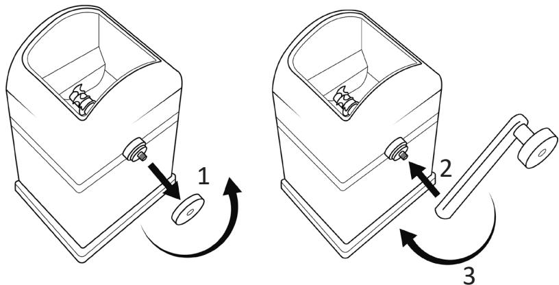
Remove the thread cover from the back of the appliance.
