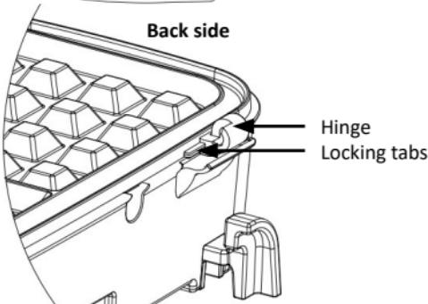
1. Insert the two plates with the locking tabs facing towards the hinge and press the plates down into the holder until they snap into place with an audible sound.
