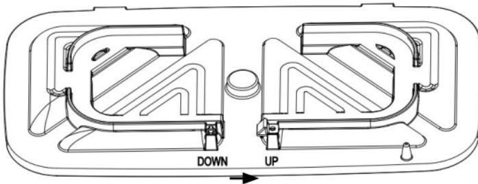
2. The lock in the "DOWN" position is for the lower plate.
