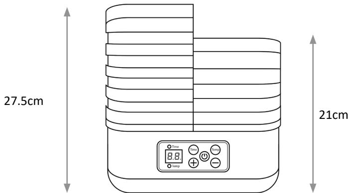
It is possible to rotate the inlay trays and the lids by 180°, thereby reducing the corresponding height.
