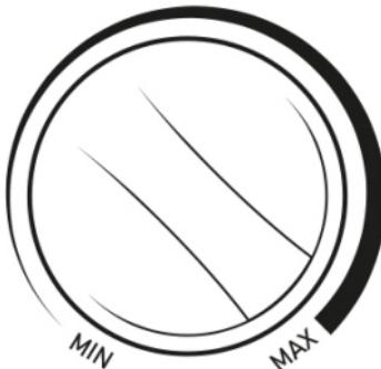
lowest temperature and "MAX" is the highest. To switch off the appliance, turn the "Temperature regulator" in the counter-clockwise direction till the appliance switches off with an audible "click".
